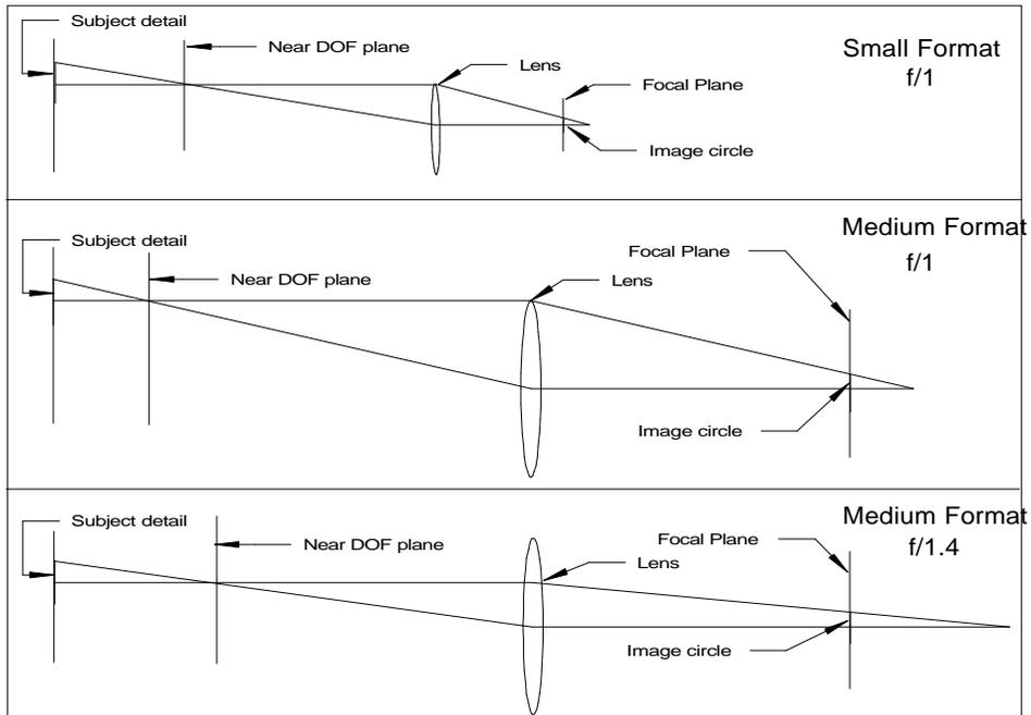
Figure 1: DOF geometry.
